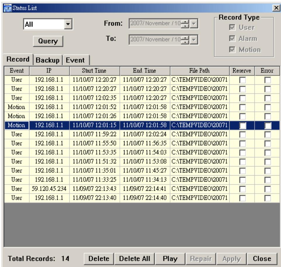
To immediately play a recording file, select a log from the list, and click “Play” button, or double-click the selected log. Then, the playback control panel will be shown at the bottom of the main control panel similar to the following.
