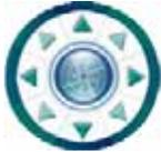
Navigation Buttons                          | Press this button to move the network camera Up / Down / Left / Right / Upper Left / Upper Right / Bottom Left / Bottom Right.                                 |
