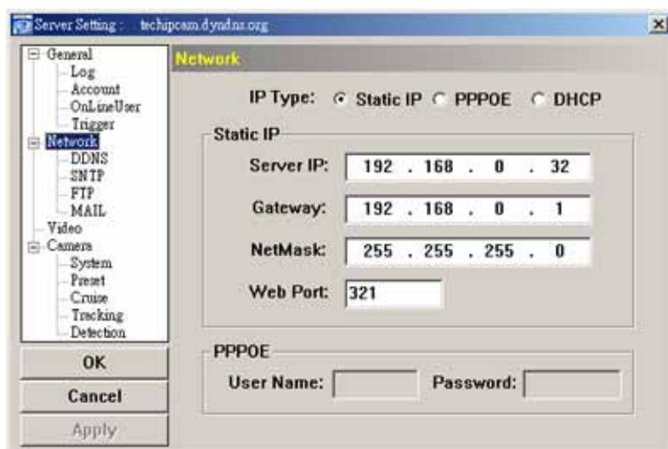
Select the network type you will be using for the network camera connection. There are 3 network connection types: Static IP, PPPOE and DHCP.
